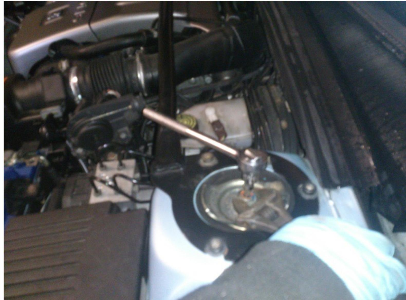
9. Unbolt and remove top shock mount torx bolts x 3. The shock will now literally just drop out of the wheel arch as an assembly, use spring compressors to take the tension of the spring and remove top mount. Old bearing will need prizing away from the inner of the top mount.
