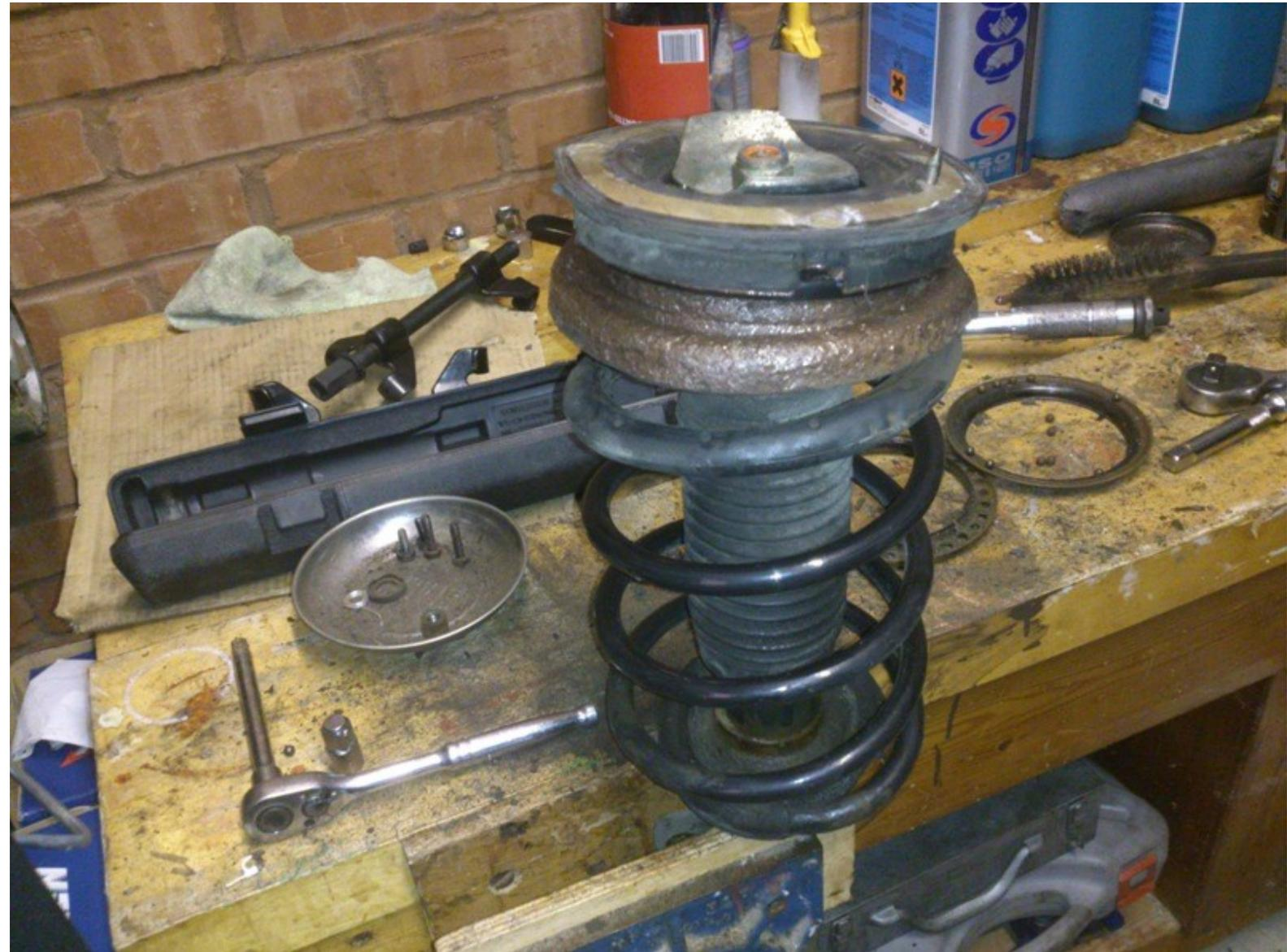
Re fitting can be awkward as someone needs to be in the wheel arch holding the shock in place whilst someone else is under the bonnet putting the 3 torx bolts back in. Also note whilst refitting the shock leave all bolts slack until its back in the hub and TRE/links are back on, you'll need this for movement. Dont forget to tighten them back up when everything in the wheel arch is back together and tight.
