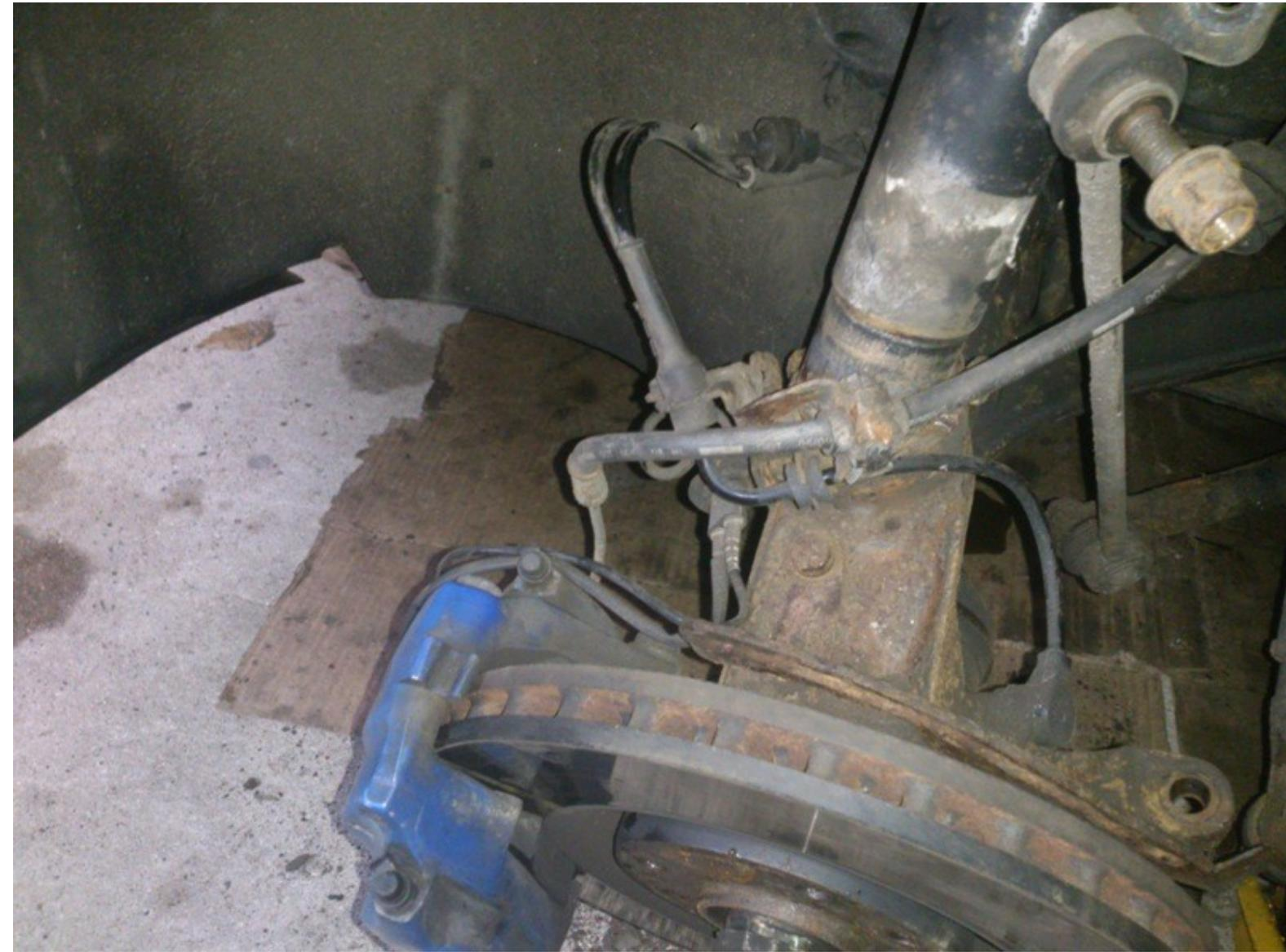
7. Undo pinch bolt that holds bottom of shock, tap or lever hub away from shock.
