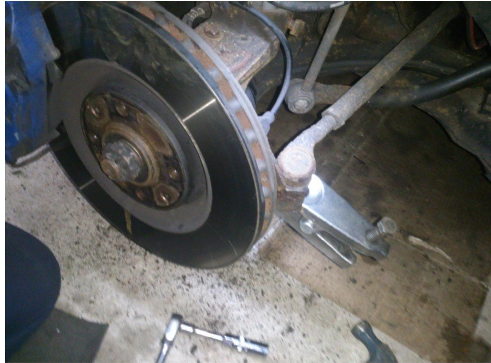
6. Unbolt cable/brake pipe tidy metal bracket holder thingy.
