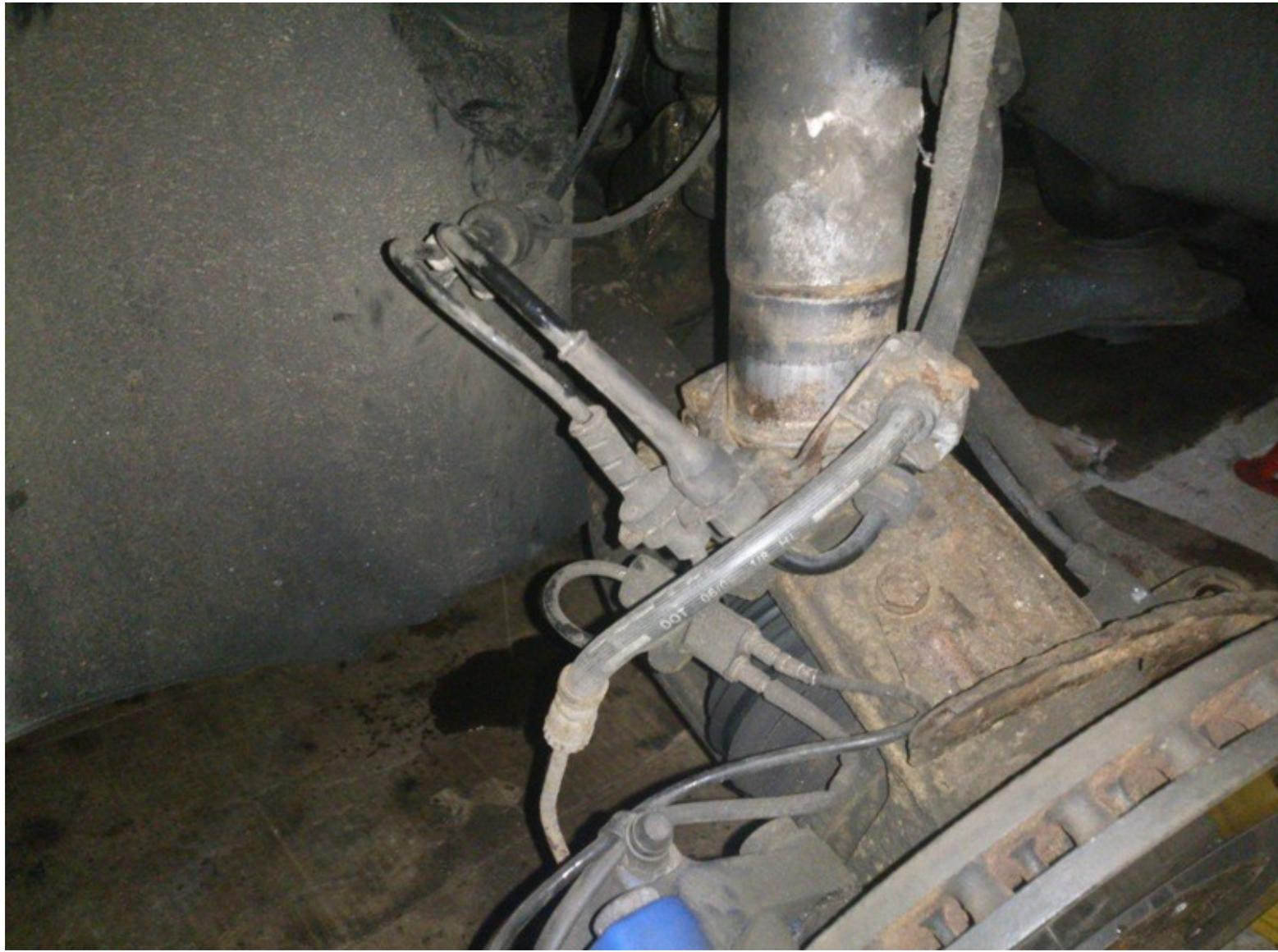
8. Slacken BUT DO NOT UNDO top shock bolt, you'll need it loose for when its off but this bolt retains the coil springs tension.
